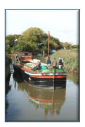
On purchase by the Society the paintwork was faded and peeling. There was no wheelhouse and all the external fitting had gone apart from the winch. The hold was full of water. After 3 years of hard work *Syntan* was completely restored to its old glory and painted in the Hodgson colours. Mast lights, engine room vents and the wheelhouse were found and fitted to their original pattern. The galley and office were created, and the hold converted into a meeting room, and living museum.
